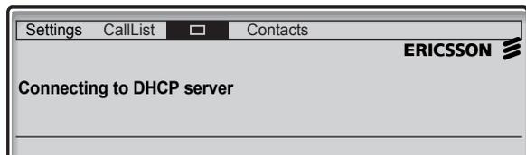
The IP telephone is connecting to the DHCP server and gets its IP address from the network.
