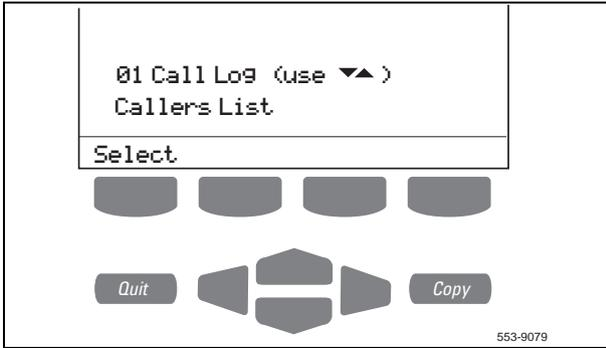
The **M3904** has a three line display. When you press the **Directory/Log** Key, the following screen appears:
