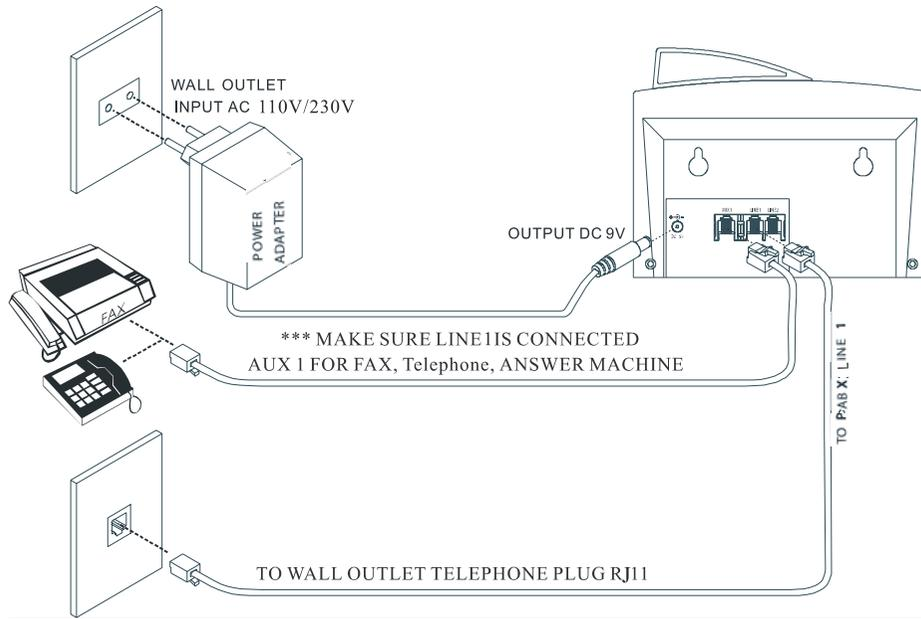
Plug one end of the adapter into the power outlet and the other end into the adapter socket on the bottom of the base.
