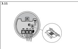
**3.11** Adjust outgoing volume with transmit volume control on base unit. Switch through the 3 settings until test person confirms the appropriate volume. <sup>1)</sup>
