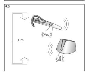
**9.3** Make sure headset and base are within 1 m of each other. When pairing is successful, both visual indicators will flash blue 5 times, and the visual indicator on base unit will turn to steady green.
