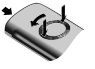
Insert a coin into the cavity at the top of the battery cover and twist it until the cover opens.
