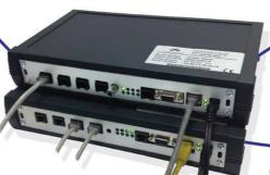
All units have a power failsafe device so if the power is lost the PSTN can still connect to the PBX and calls can still be made
