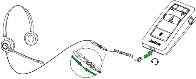
If the headset is QD disconnected during a call, the call will be put on audio-hold. Reconnecting the QD resumes the conversation.
