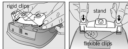
Insert the rigid clips of the stand into the slots on the bottom of the phone (near the ringer cover). Press down firmly until the flexible clips clicks into place.
