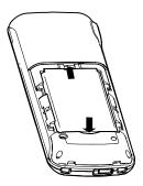
Replace the battery compartment cover back on the phone. Slide the battery compartment cover upwards until it snaps in to place.
