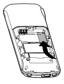
Insert the battery. The golden contacts on the battery must face towards the top left. Press lightly on the bottom end of the battery until it snaps into place.
