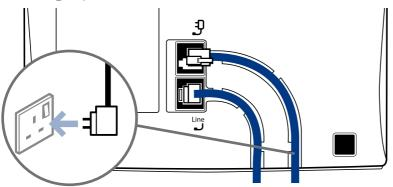
Plug the mains power adaptor (item code 039956) into the socket marked 9 on the underside of the base and plug the other end into the mains power wall socket and switch the power on.
