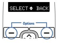
If no button is pressed for 30 seconds, the handset returns to standby automatically.
